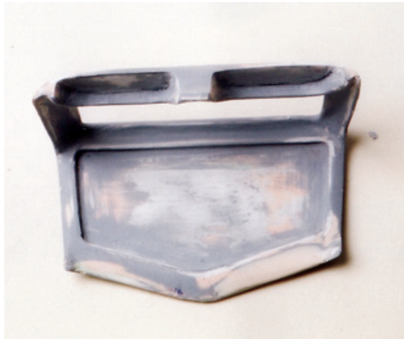
Figure 7.46: The process of readying this part for final painting requires a lot of shaping, putty, sanding, more catalyzed putty, primer and more sanding, all while constantly checking the fit of this part to the inside of the cab roof. As this work progresses, this part is repeatedly placed into the cab to check for fit. Note that small protuberances have been added at the outside corners of the front of the headliner insert, and will eventually locate the upholstered panels that fit inside the A pillars.
