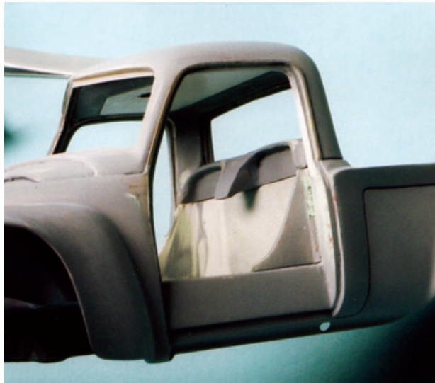
Figure 7.50: The seat surround, shown in its early stage, is placed inside the cab and beneath the headliner/rear window insert. Note how the shape of the upper seat receiver will sweep up and around and follow the side of the seat. Eliminating or minimizing the part-mating line between these two parts will be a challenge; either a piece of trim to cover the interface or a very tight line will be necessary. Again, prepare an assembly manual to govern construction; there is only one sequence that allows the interior of the DT 2 to go together.
