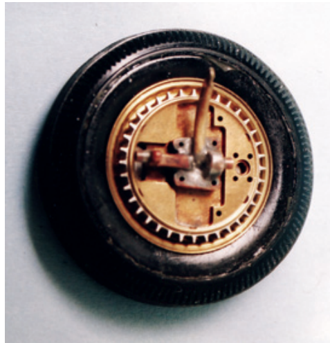
Figure 7.4: The cast and machined spindle is index-drilled to exactly match the Bendix brake backing plate that fits closely into the drum brake which, in turn, matches the bolt pattern of the rim. The taper on the OD of the brake backing plate matches the taper on the ID of the Buick brake drum to insure a fool-proof, same-every-time fit. Compare this photo to Figure 7.3.
