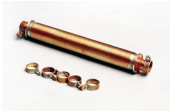
Figure 7.42: The tubular mufflers will mount inside the frame rails and will “hang” on the small machined/soldered brass “hangers.” Those clamps will be attached to photoetched hangars insulated by “rubber” straps “bonded” to a bracket that will be bolted to the frame. Of course, the diameters of the inlet and outside muffler clamps, as well as the hangers, match commercially-available brass tubing. Since DT 2 will be built as a “show truck,” all chassis-mounted exhaust parts will be nickel plated, and the lake pipes will be chrome plated.
