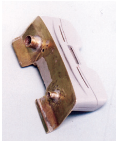
Figure 7.37: The Lynx dashboard is located to the body using positive mounting points to assure stability and predictability of how parts fit in two ways: a brass sleeve for the heater motor that fits into a sleeve placed in the firewall, and the console (not shown here) that fits up under the center part of the dash which, in turn, pins to the transmission tunnel. Note that defroster vents, the cut-out for the speaker, and the line that will define the painted and padded parts of the dash top.
