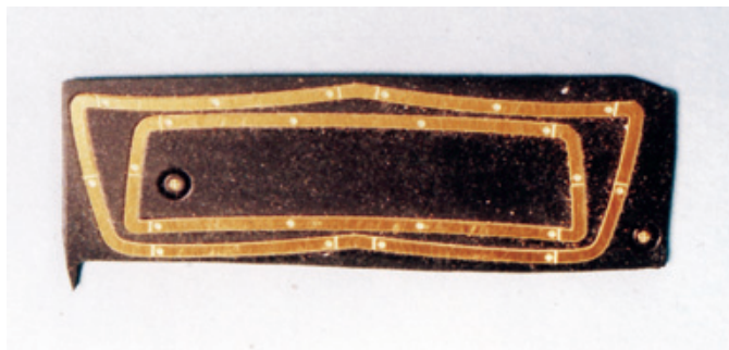
Figure 7.56: Mirror-image photoetched trim parts were drawn by Bob Wick and photocut by Fred Hultberg. Note the “cut lines” which delineate where the several parts that make up a trim set would exist in this application. Note also here the ultra-small Phillips-head screw relief cuts because inside trim is most usually secured by screws. When polished, this trim will be nickel plated (because none of this trim, as anodized aluminum or polished stainless in 1:1 scale, would have a “blue”-chrome appearance).
