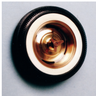
Figure 7.5: Flipped over, the rim (complete with the center cone and spinner) fits tightly into the Modelhaus tire. Compare this image to Figure 7.2.
