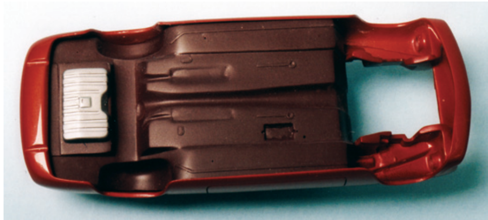
Figure 7.12: . . . into its final position in the body. More work could have been done to widen the rear wheelwells to fit more tightly into the inside of the rear quarter panels. Now, the modified kit frame attaches to the underbody.
