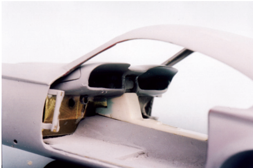
Figure 7.38: The plastic dash is permanently affixed to a brass structure that not only provides a stable and secure mounting surface for the dash, but also creates a smooth toeboard for the cabin. This view also shows the console in place.
