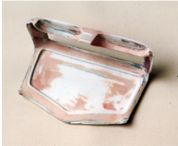
Figure 7.45: Because the cab and floor are one assembly, it's essential to create an "insert" that will serve as the molded headliner and adjoining "upholstered" panel. To do that, a part comprised of the headliner, a panel around the rear window, and pieces that fit down inside the B pillars and will serve double-duty as the "receivers" for the seat inserts is created from multiple pieces of .040 sheet styrene. The center of the headliner will receive a pleated insert.
