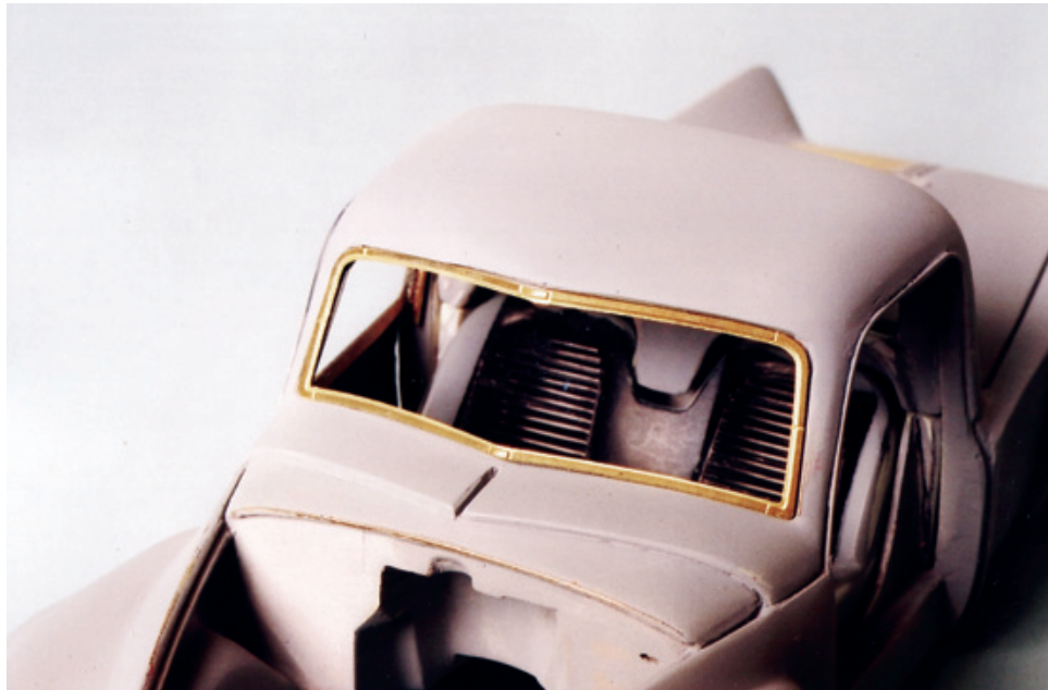
Figure 7.55: The exterior trim was photoetched, with double-cut lines placed in the trim to simulate the likely length of each piece of the multi-piece assembly that comprises windshield trim.
