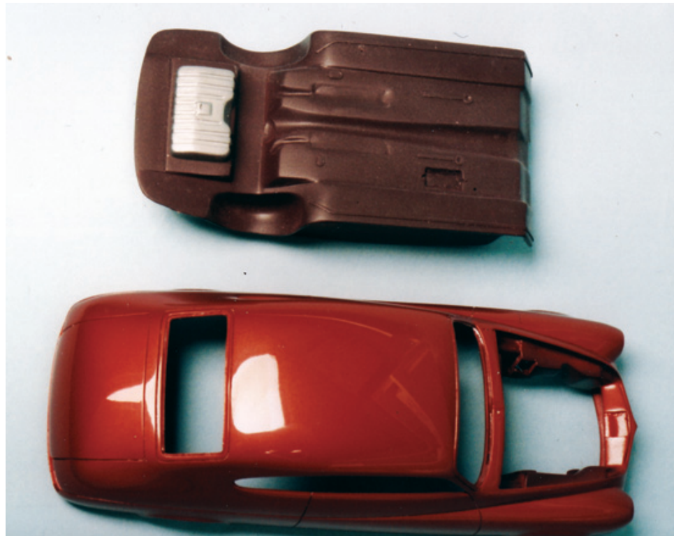
Figure 7.9: The other way to create a realistic body-on-frame model, when you don't want to open the doors, is to mate the interior tub to the floorboard to the bottom of which the frame will be placed. On the New Age Merc , this technique was tried successfully but note that the frame still had to be cut loose from the kit floorboard to achieve this method of construction.
