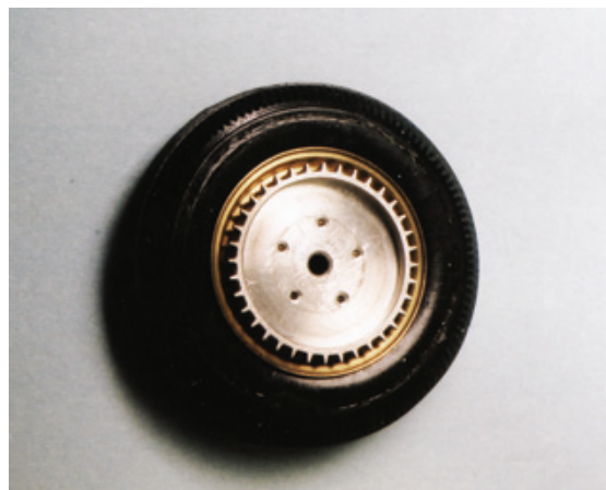
Figure 7.3: From the backside, note the carefully-managed tolerances between the outside diameter of the Buick brake drum and the inside diameter of the rim. There is a sleeve on the fascia of the spindle that indexes into the back of the brake drum.
