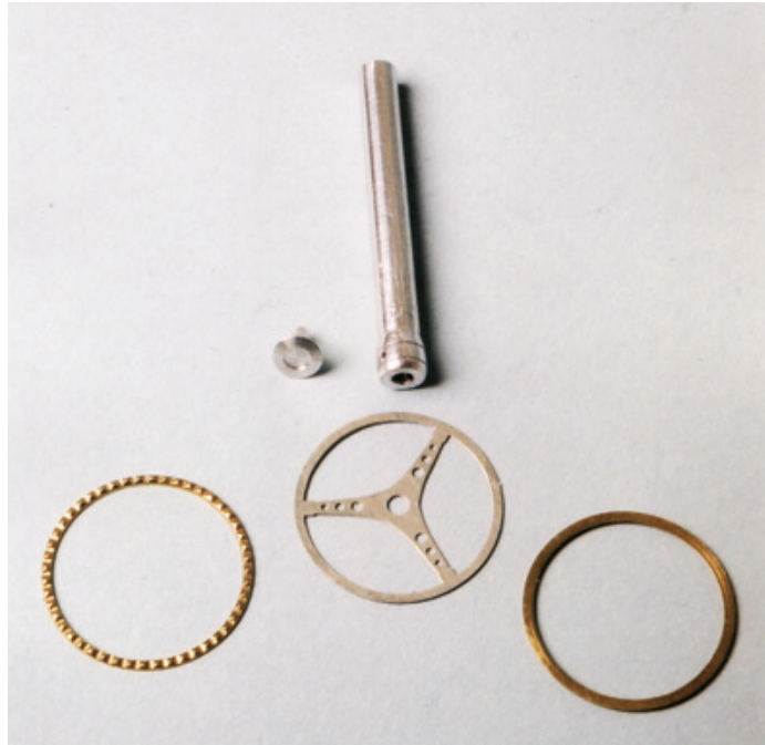
Figure 7.43: The steering column and Corvette steering wheel for DT 2 generally mimic the steering wheel from the pre-accident version of Spencer Murray's Dream Truck . The length of the column and its diameter, as well as the dimensions of the steering wheel and the spoke detail, were all taken from 1:1 scale parts.
