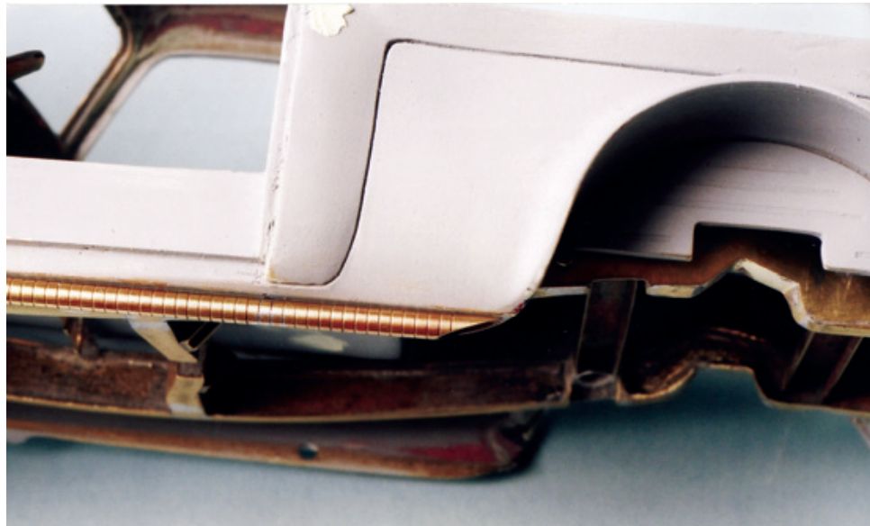
Figure 7.41: Note the concentric rings on the exhaust pipe that match the rings on the front and rear grille work, and note how the curvature at the end of the pipe matches the sweep of the rear wheelwell flare. Think about the interface between styling and function. With the frame in place, the exact relationship between the parts can be identified early, meaning that the final assembly of the exhaust system will go smoothly.
