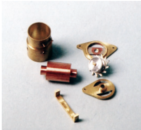
Figure 7.31: Similarly, the generator ( Dream Truck 2 is built to 1961 mechanical standards) is a multi-part assembly, and everything goes together easily. The armature was turned from copper to simulate the armature windings when it is seen through the small “windows” in the generator housing.
